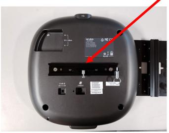
All AP-5xx will ship with the Common Mount pre-attached (to minimize risk of customers damanging threads and to make new installs easier)
